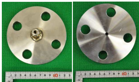
Fig. 4 Appearance of general-purpose 25A flange
