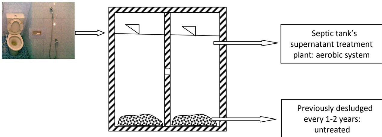
Fig. 4.1 The RSUD Wonosari wastewater treatment plant diagram
