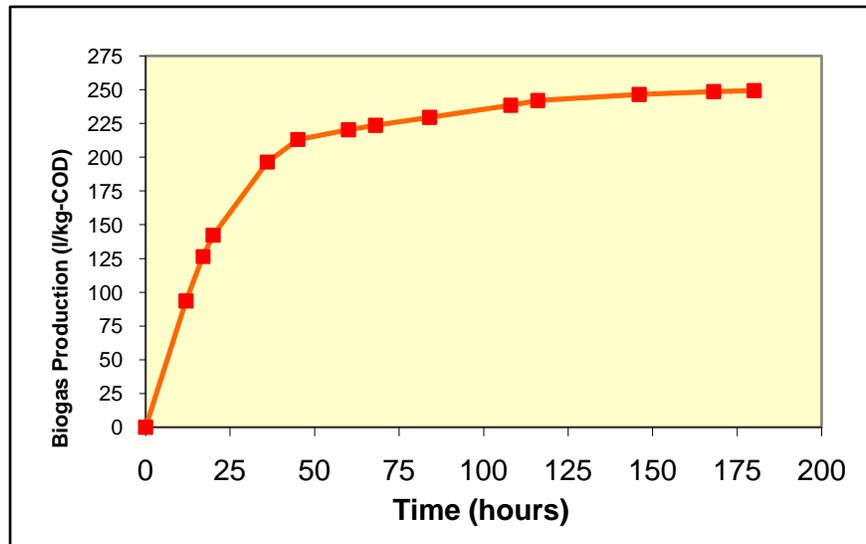
**Fig. 4.2** Net Biogas Production Potential of Septic Tanks' Sludge
