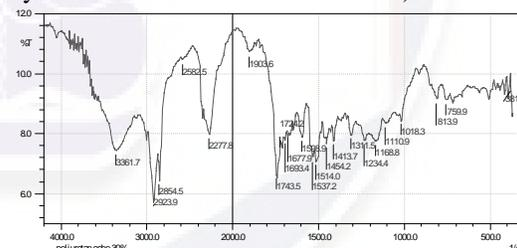
Fig 3. The FTIR Spectrum of PU Based Oxydated SBO - MDI
