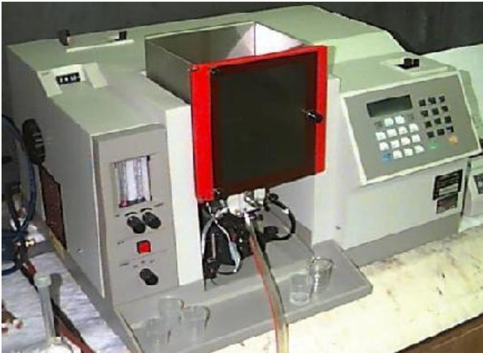
*Picture of a flame atomic-absorption spectrometer*
