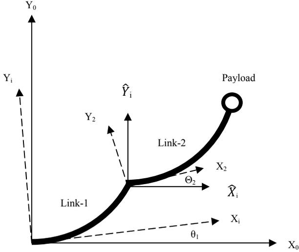
**Figure 1.** Structure of a two-link flexible manipulator
