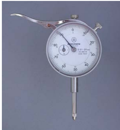
Gambar 1.8. Jam ukur ( Dial Indicator )
