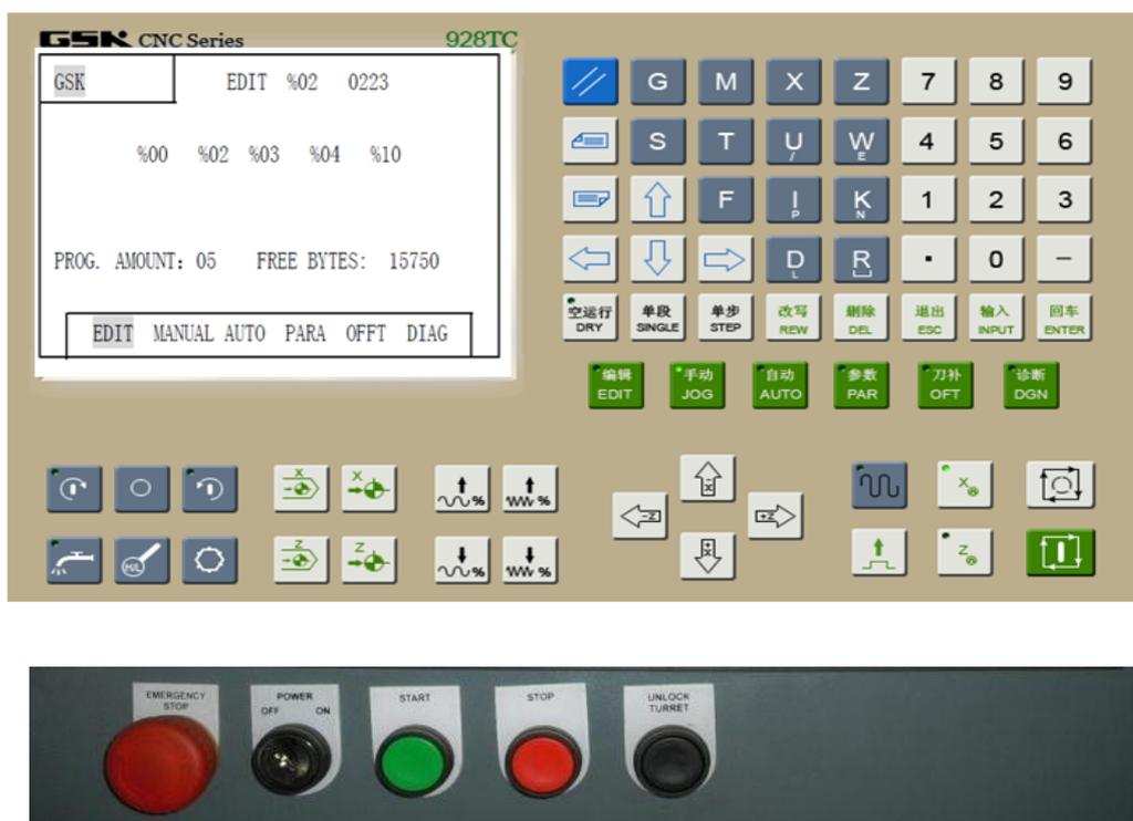
Gambar 2.27. Panel kontrol mesin Frais CNC GSK 928 TE
