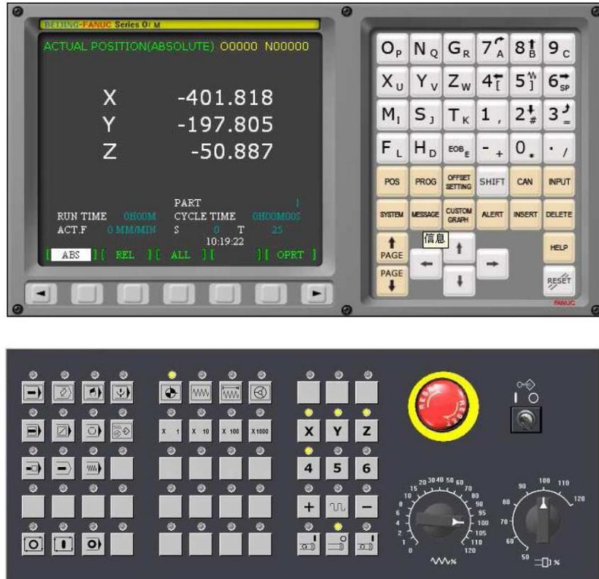
Gambar 2.26. Panel kontrol mesin Frais CNC Fanuc OiM
