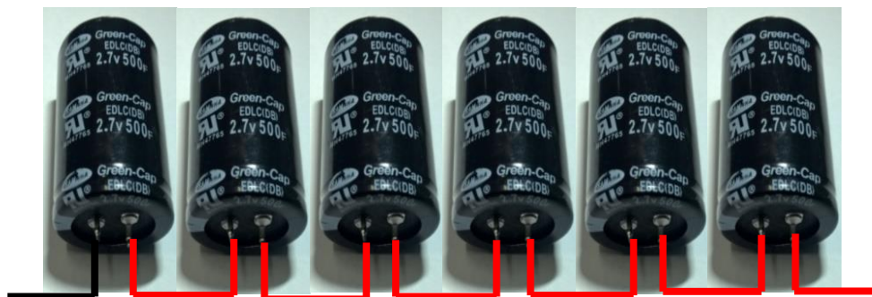
Figure 2. Series arrangement of six supercapacitor 500F/2.7voltage
