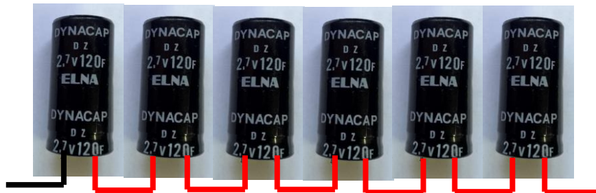
Figure 1. Series arrangement of six supercapacitor 120F/2.7voltage
