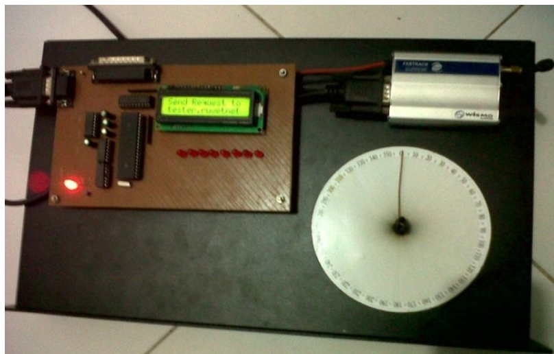
Gambar 1 : Led 8 bit dan motor stepper sebelum nilai website “ tester.ruwetnet.com ” di update
