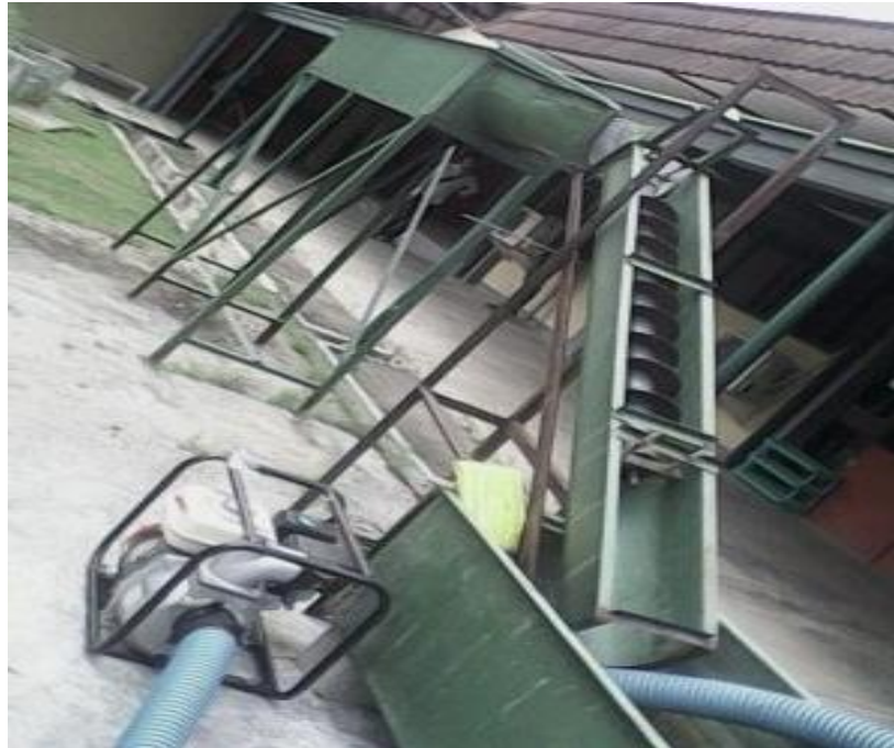
Gambar 3 Apparatus Pengujian Kincir Air Screw
