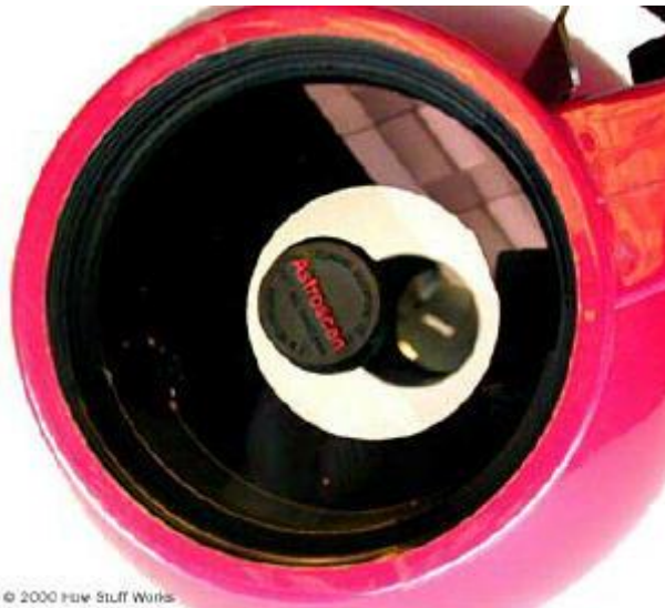
A view inside the barrel — note the primary mirror, and the image of the secondary mirror reflected back onto the primary.
