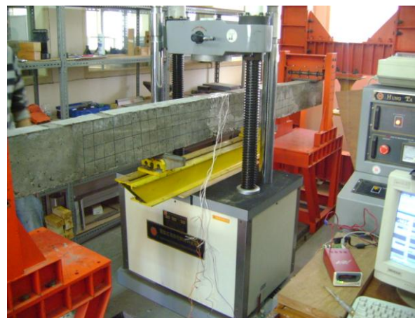
Figure 2. Experimental set-up with computerized UTM and data logger of strain gauges (Susilorini, 2009b)
