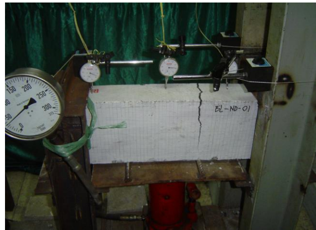
Figure 6. Cracked deep beam using nylon mesh confinement (Lelono and Widi, 2009)
