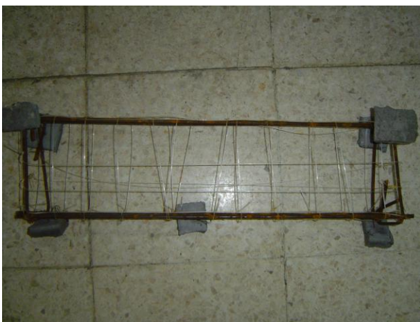
Figure 1. The placement of nylon mesh confinement for deep beams which cover the steel bar (Lelono and Widi, 2009; Susilorini, 2009a,b)
