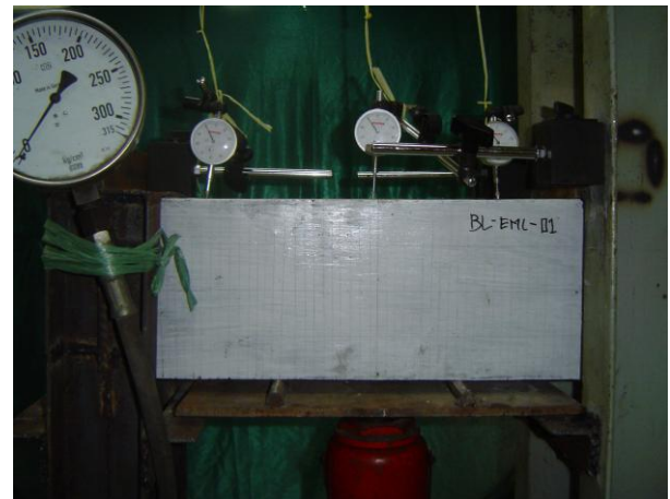
Figure 3. Experimental set-up with dial gauges and hydraulic jack loading equipment (Lelono and Widi, 2009; Susilorini, 2009a,b)
