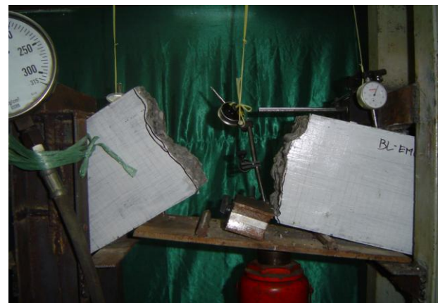
Figure 7. Failure of deep beam using expanded metal sheet confinement (Lelono and Widi, 2009).
