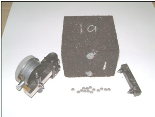
Figure 5. The CDWblock sample and strain measuring equipment
