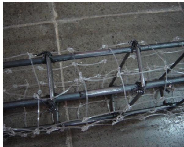
Figure 1. Nylon mesh with mesh spacing of 5 cm which cover the steel bar (Susilorini, 2009b)
